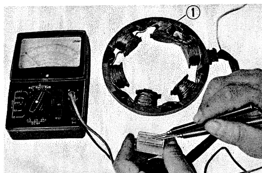
Fig. 152 Stator coil test ① Stator coil
